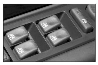
The controls for the power windows are located on the armrest on each of the side doors. The switches operate the windows when the ignition is in RUN, ACCESSORY or when Retained Accessory Power (RAP) is active. See "Retained Accessory Power" under *Ignition Positions on page 2-18*.
